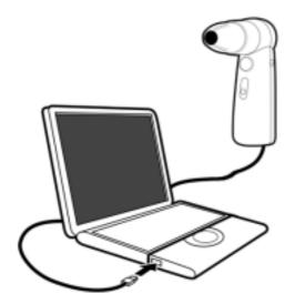
Plug the connector of the USB Microscope into the PC USB port.
